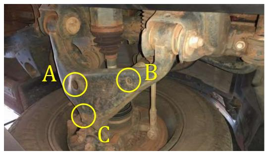
• Hole C also has a hole on the top of the control arm where the M10 threaded bush fits to secure the M10x60 countersink bolt.
